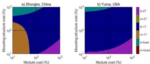
Figure 4. Stability of the results exemplarily calculated for one location in China (Zhongba) and the US (Yuma), exemplarily. The plot shows in color which system configuration is preferable as a function of module cost and mounting structure cost.
