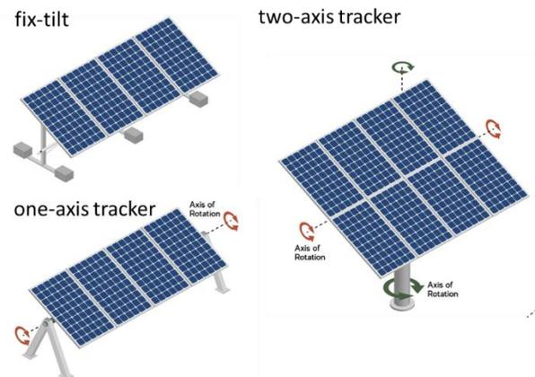
Figure 1. Different system configurations explored in this study. Figure reprinted from [8].
