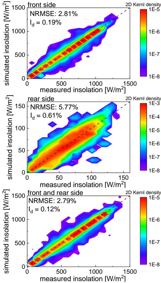
Figure 2. Comparison of simulated and measured irradiance at front, rear and for both planes simultaneously of a horizontal single axis tracking installation. Plotted are the 2D kernel densities of the comparisons.
