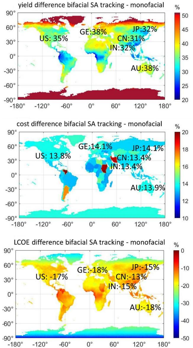
Figure 3. Comparison of techno-economic parameters (yield, overall system cost, LCOE) between a single-axis (SA) fixed tilt installation and a one-axis tracking installation with bifacial PV modules. Exemplary values are given for, west to east, the US, Germany (GE), India (IN), China (CN), Japan (JP) and Australia (AU).
